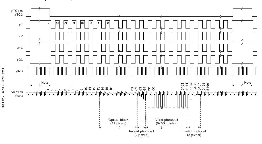
**Note** Input the  $\phi$  RB pulse continuously during this period, too.
